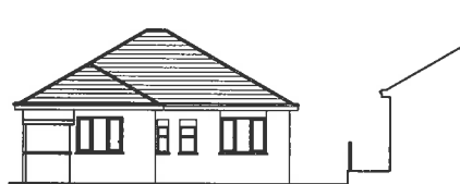
EXISTING REAR ELEVATION. SCALE 1:100
